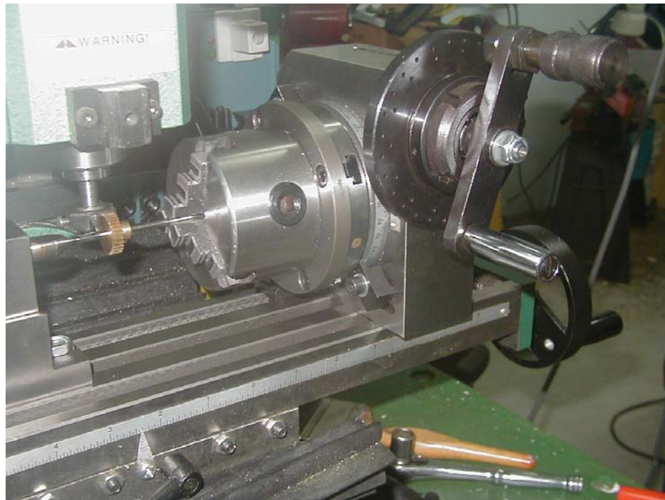
The rotary table setup horizontally with 3-jaw chuck and dividing plate.
