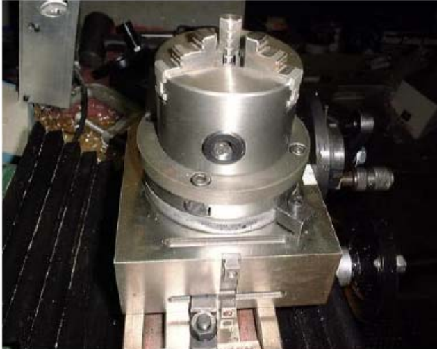
Lathe chuck mounted on a rotary table (mounted vertically)
