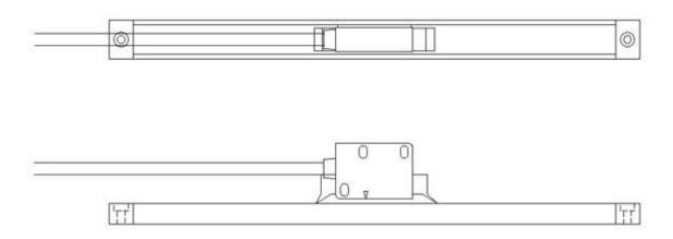
Use the provided M3 screws to mount the reader heads. Use a 2.5 mm or #39 tap drill and an M3x0.5 metric tap.
