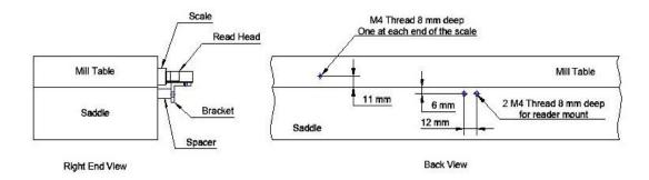
In most cases, the reader can be mounted at the center of the saddle with the scale symmetrically mounted on the table. But on some very small machines there's not enough room between the saddle and the column so the reader must be mounted off center, with the scale also mounted off center.
