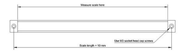
Place the channel in a vise with the "U" facing up and your mark just off the side of the vise. There is a thin strip of stainless steel protecting the magnetic strip in the channel. Using the finest hacksaw blade (or band saw blade) you have (preferably 32 teeth per inch), carefully saw down through the channel.
