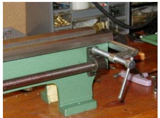
with the left end of the way casting. Use a small C-clamp on the top ear of the bracket to hold it in position.
