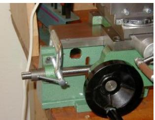
screw mounting bracket in the correct position.
